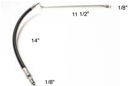
POWER TRIM HOSE Port • Connector to bottom of trim cylinder MCM 120-260 & BRAVO
