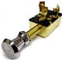
MP39570** MP39572 (Bulk 100pcs/carton) OFF-ON(1)-ON(1&2) SPDT • First pull energizes #1 • Second pull energizes both circuits • Solid brass construction • 3/8" mounting bushing • 3 screw terminals • For panels up to 1" thick • Chrome finish plastic knob • Rated: 15 amp @ 12 VDC
