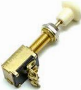
MP39510 MP39512 (Bulk 100pcs/carton) OFF-ON SPST • Pull for ON • Solid brass construction • 3/8" mounting bushing • 2 screw terminals • For panels up to 1" thick • Cream plastic knob • Rated: 15 amp @ 12 VDC
