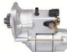
18-6931 STARTER Replaces: Yanmar 119209-77010, 121120-77010, 77011, 77012, 124520-77010, 77011 Fits: 3 TNV-84-T engines
