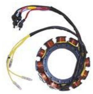
18-5871 STATOR Replaces: 398-5454A32 For: 135-300 V6
