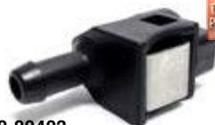
18-80403 FUEL CONNECTOR Female 3/8 hose connector with rectangular locking post, Will not interchange with OE's 5/16" hose assemblies. For late model engine: For use with our 18-81042 fuel hose assembly, motor end. Mates with 18-80407
