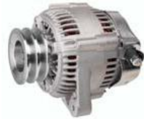
18-6849 ALTERNATOR Replaces: Yanmar 119773-77200 Denso 101211-9940 Fits: Yanmar Engines
