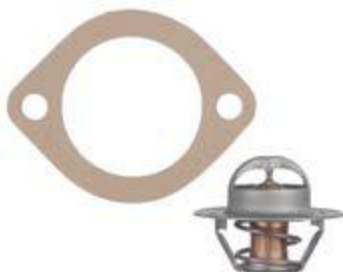
23-3661 THERMOSTAT KIT Replaces: Westerbeke 35736, 40434 Temperature Rating: 140° Fits: 20.0 BEG(60Hz)/16.0 BEG(50Hz), 25.0 BEG(60Hz)/20.0 BEG(50Hz)
