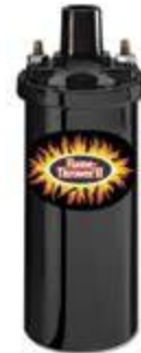
18-5472 HI-PERFORMANCE IGNITION COIL 0.6 ohm (oil filled), black - 4, 6, & 8 cylinder: Flame-Thrower 45,000 volt coil. ★ Super low 0.6 ohm resistance coil designed for use with the Ignitor II Hi Performance Electronic Conversion Kits ★ Compatible with capacitive discharge systems
