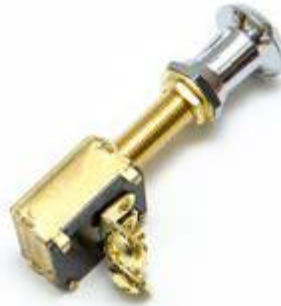
MP39520** MP39522 (Bulk 100pcs/carton) OFF-ON SPST • Pull for ON • Solid brass construction • 3/8" mounting bushing • 2 screw terminals • For panels up to 1" thick • Chrome plated plastic knob • Rated: 15 amp @ 12 VDC
