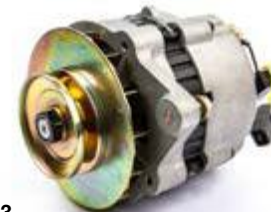
18-6263 ALTERNATOR Replaces: 288182, 288759 12 Volt, 51 Amp, Integral Regulator, Negative Ground, Single Groove Pulley For: Universal and others (I/O)
