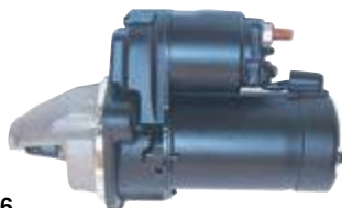
18-5906 STARTER Replaces: 840808, 872241 • Inboard • Gear Reduction Starter • Permanent Magnet, 12 Volt • CW Rotation • Aluminum Pinion Housing w/2 Threaded Mounting Holes Fits : Volvo Penta 4 Cylinder and 6 Cylin- der Gas Engines
