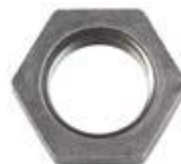
18-3719 PINION NUT Replaces: 11-35921, 11-47411, 11-826375, 11-F694188 5/8" - 18 thread • 1 1/16" wrench
