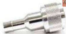
18-80401 FUEL CONNECTOR Female hose connector, new style, 3/8" hose, Will not interchange with OE's 5/16" hose assemblies. Mates with 18-80400 , tank outlet
