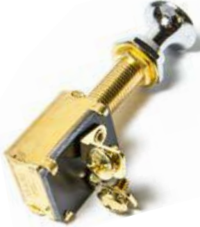
MP39530** MP39532 (Bulk 100pcs/carton) OFF-ON SPST • Pull for ON • Solid brass construction • 3/8" mounting bushing • 2 screw terminals • For panels up to 1" thick • Chrome plated solid brass knob • Rated: 15 amp @ 12 VDC
